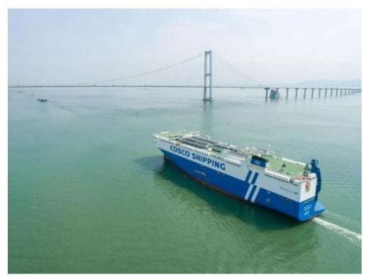
On May 15, the LNG dual-fuel car carrier "YUAN HAI KOU", a fleet addition by Guangzhou Yuanhai Auto Carrier—a subsidiary of COSCO SHIPPING Specialized—undertook its maiden voyage from the Nansha Auto Port in Guangzhou. Stretching 199.9 meters in length and equipped with 12 car decks (4 of which are adjustable), the "YUAN HAI KOU" is designed to accommodate a diverse array of vehicles, including commercial trucks, engineering machinery, buses, and MAFI cargo.
