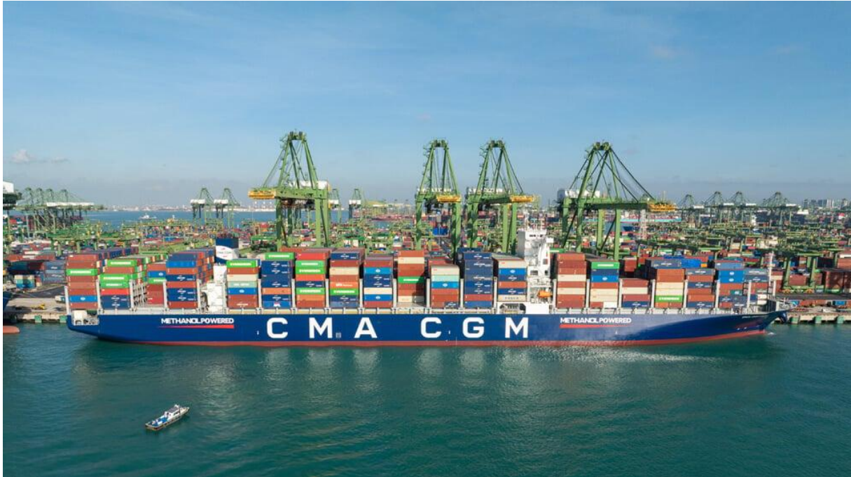
CMA CGM Iron is the first of a new class of a dozen methanol-fueled containerships (CMA CGM)
