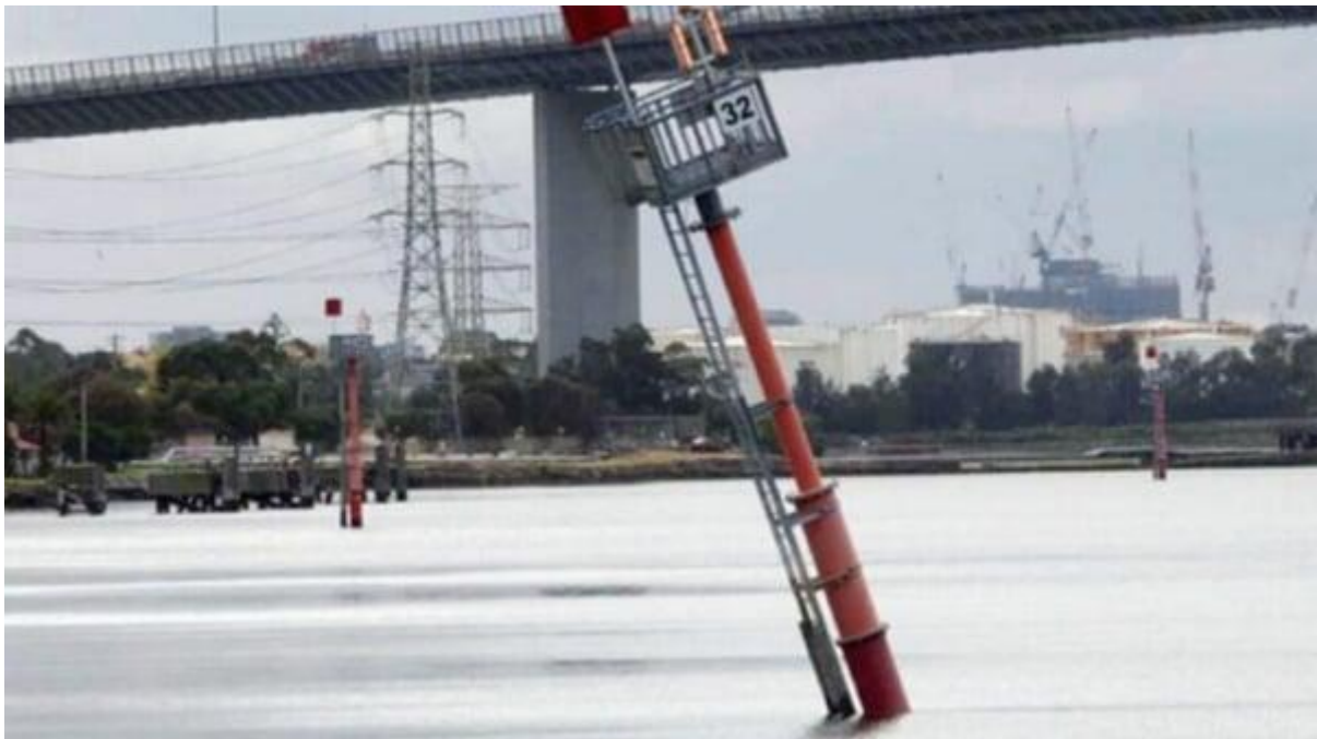
CMA CGM Puccini severely damaged the beacon while departing Melbourne, Australia (ATSB)
