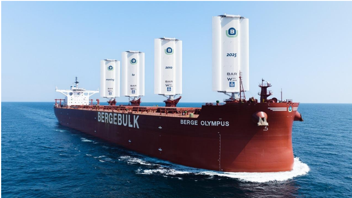
Berge Olympus fitted with wind assisted propulsionCredit: Berge Bulk
