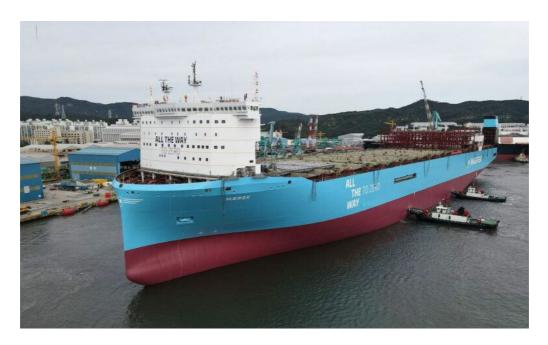
Maersk has revealed the design of its new-look series of 16,200 teu methanol-fuelled ships which feature the accommodation at the bow and no islands along the vessel.
